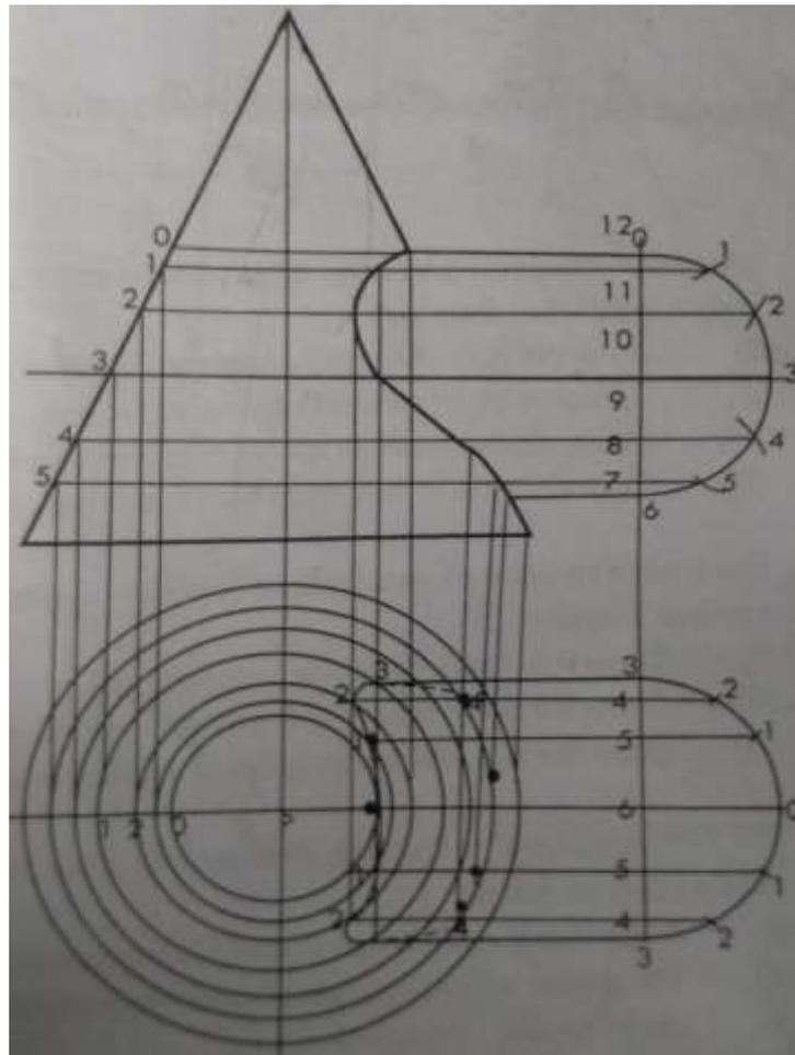
5. To draw the curve of intersection of two unequal cylinders, indicating the surface development of the smaller cylinder from the front elevation and section in plan of a similar cylinder on the plan.
