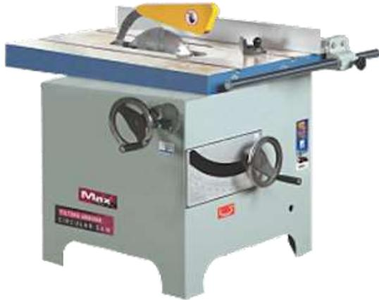
The circular saw is used to prepare or resaw timber into suitable sizes for articles of joinery, furniture and some other items made of wood. This machine has a table, with a revolving knife protruding above the table.
