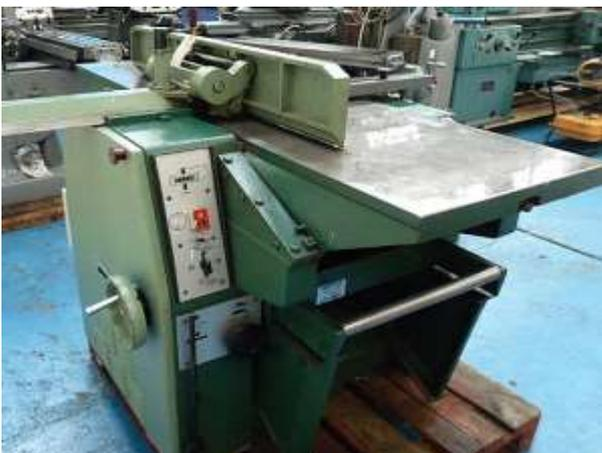
The thicknesser is a woodwork machine used for planing to a specific thickness. It is similar to the surface planer. This machine is used to produce correct thickness by setting the cutter to the desired size.
