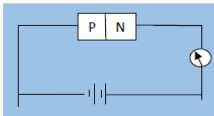
Connecting the negative terminal of the battery to the p-region and positive terminal to the n-region gives a reverse bias. The negative terminal repels electrons from p-region to n-region and positive terminal repels holes from n-region to p-region, but there are few free electrons in the p-region and very few holes in the n-region. As a result, the current in the reverse direction is much smaller than that with the same potential difference in the forward direction.
