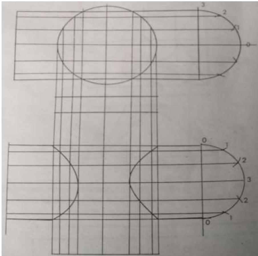
3. To determine the point of intersection of square prism intersecting a hexagonal prism.
