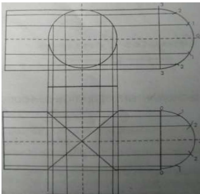
2. To construct the plan of interpenetrating cylinders.
