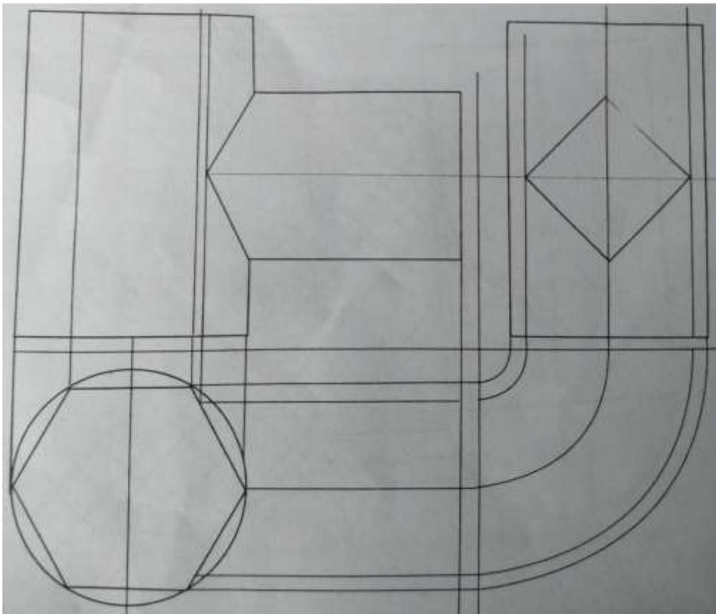
4. To determine the curve of intersection of a cylinder intersecting a right cone.
