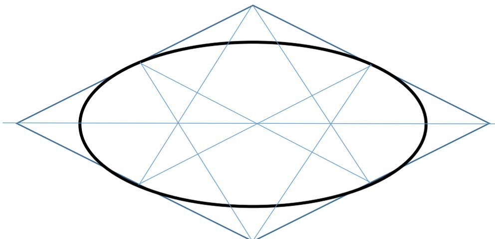
To construct an ellipse using the rectangular or geometrical method.
