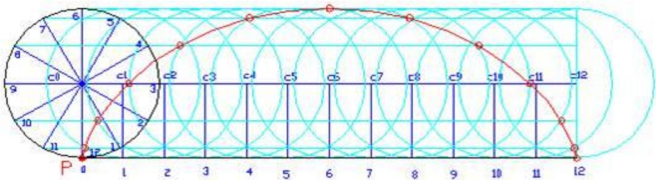
The construct of trochoid is the same with cycloid, except that we have superior and inferior trochoids.
